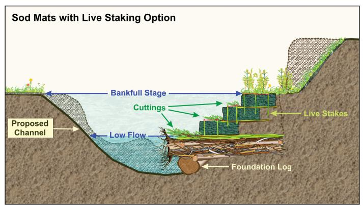
Figure 15. The toe wood structure with cuttings, sod mats and live staking.
