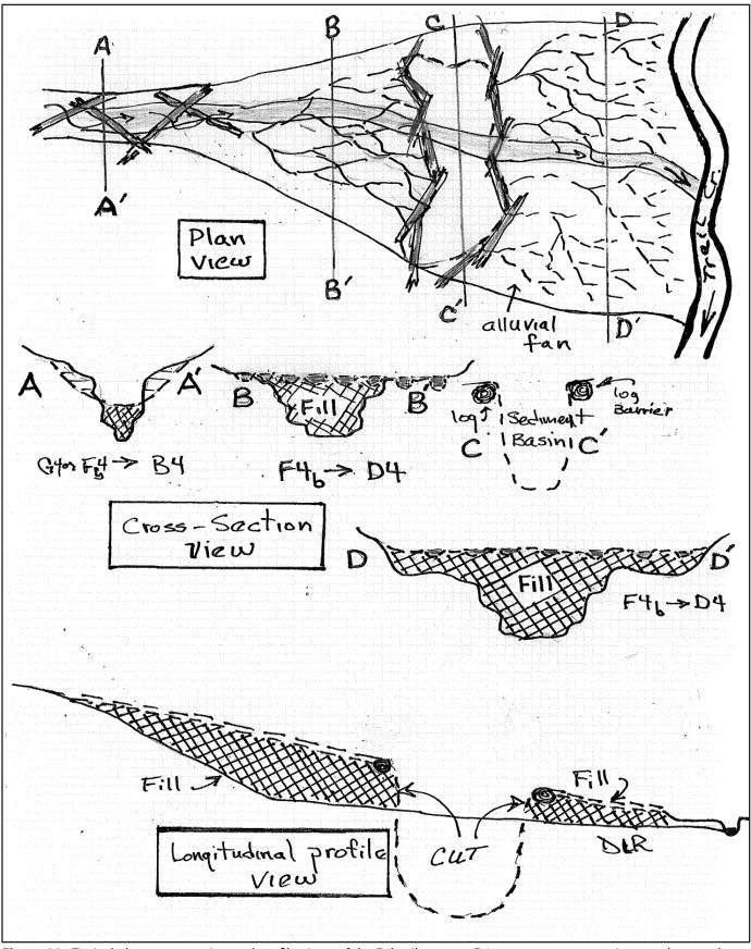
**Figure 33.** Typical plan, cross-section and profile views of the F4b tributary to D4 stream type conversion on a long and wide alluvial fan (Valley Type III) with a sediment detention basin.
