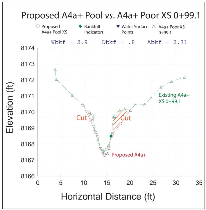
**Figure 106.** The overlay of the existing cross-section 0+99.1 *vs*. proposed pool cross-section indicating the cut and fill recommendations for the A4a+ *Poor* to A4a+ *Stable* step–pool conversion.
