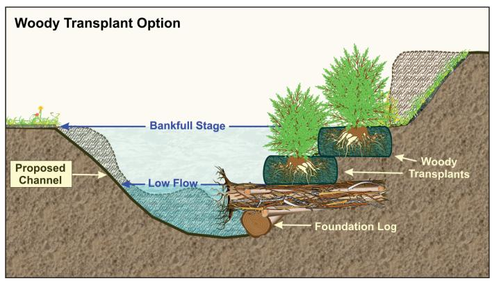
Figure 16. The toe wood structure with woody transplants.
