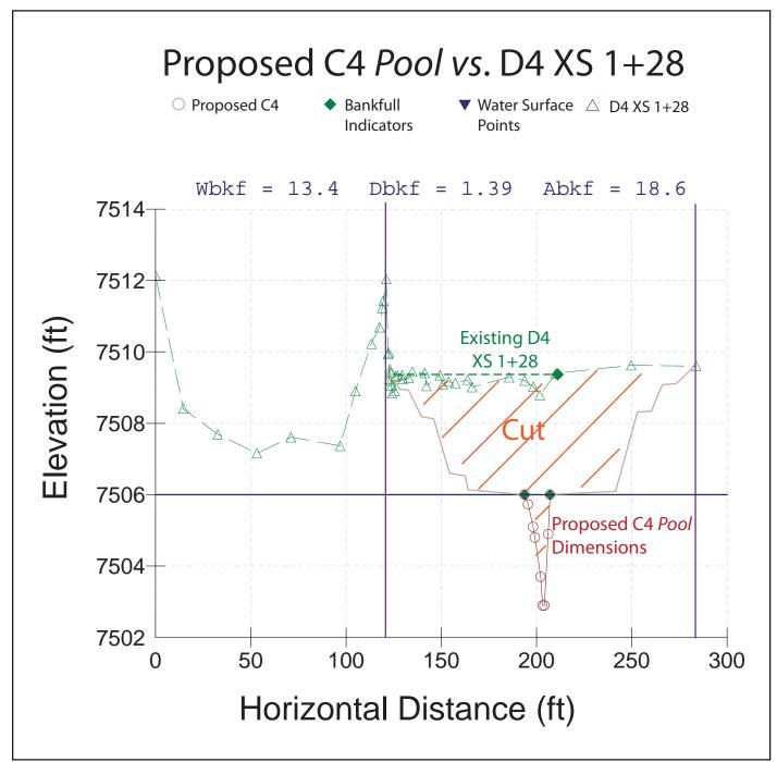
Figure 54. The proposed C4 pool cross-section compared to the existing D4 cross-section 1+28 below the West Creek road.
