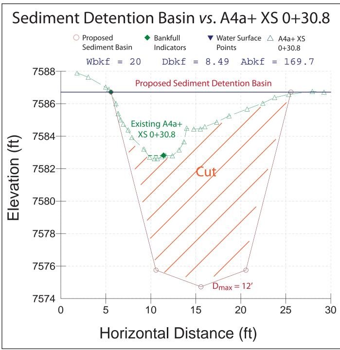
Figure 114. The proposed sediment detention basin located at the existing A4a+ cross-section 0+30.8.
