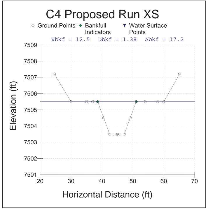
Figure 52. The typical run cross-section for the proposed C4 reach below the West Creek road.
