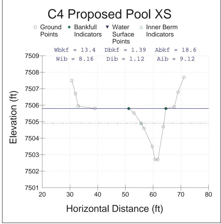
Figure 50. The typical *pool* cross-section for the proposed C4 reach below the West Creek road.
