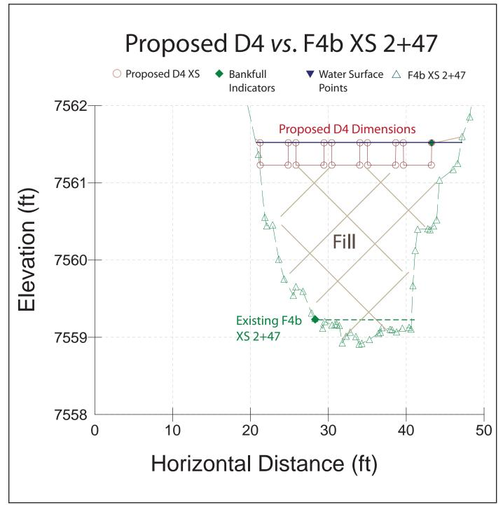
**Figure 94.** The typical, proposed D4 cross-section dimensions compared to the existing F4b cross-section 2+47, indicating the extensive fill requirements and new bankfull elevation.
