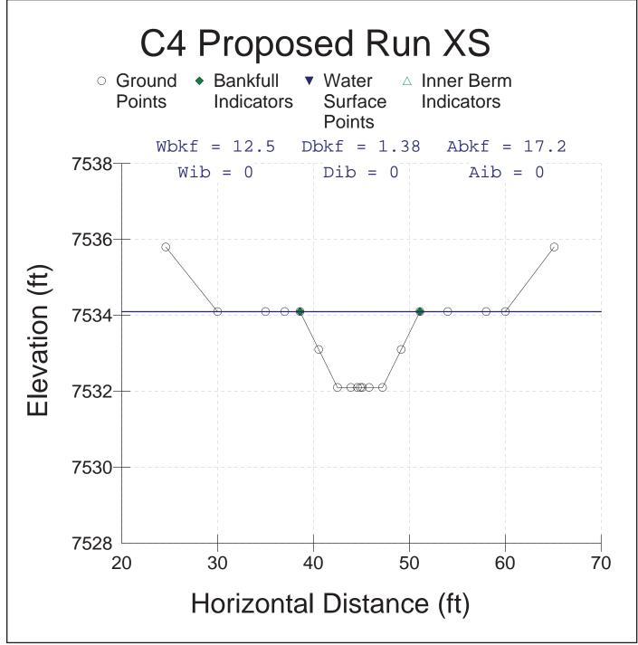
**Figure 86.** The typical *run* cross-section for the proposed C4 *Stable* design converted from the existing C4 *Poor* condition stream type.
