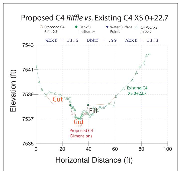
**Figure 83.** The proposed C4 *Stable riffle* cross-section compared to the existing C4 *Poor* cross-section 0+27 showing the cut and fill recommendations and reconnecting the channel with the floodplain.
