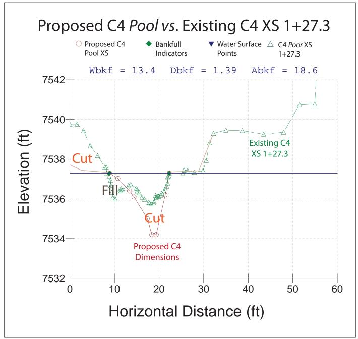
**Figure 84.** The proposed C4 *Stable pool* cross-section compared to the existing C4 *Poor* cross-section 1+27.3 showing the cut and fill recommendations and reconnecting the channel with the floodplain.
