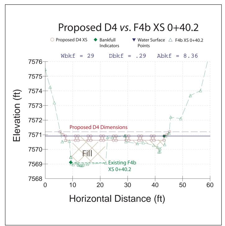
**Figure 92.** The typical, proposed D4 cross-section dimensions compared to the existing F4b cross-section 0+40.2, indicating the extensive fill requirements and new bankfull elevation.
