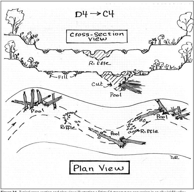
**Figure 34.** Typical cross-section and plan views illustrating a D4 to C4 stream type conversion in an alluvial fill valley (Valley Type VIII), and the proposed streambank stabilization and fish habitat structures by typical location.
