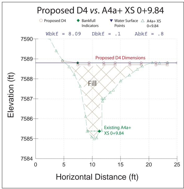
**Figure 113.** The proposed D4 cross-section *vs*. the existing A4a+ cross-section 0+9.84 indicating the extensive fill requirements.
