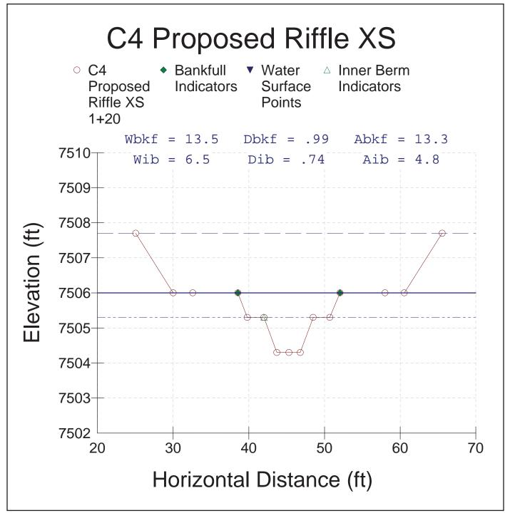
Figure 49. The typical *riffle* cross-section for the proposed C4 reach below the West Creek road.
