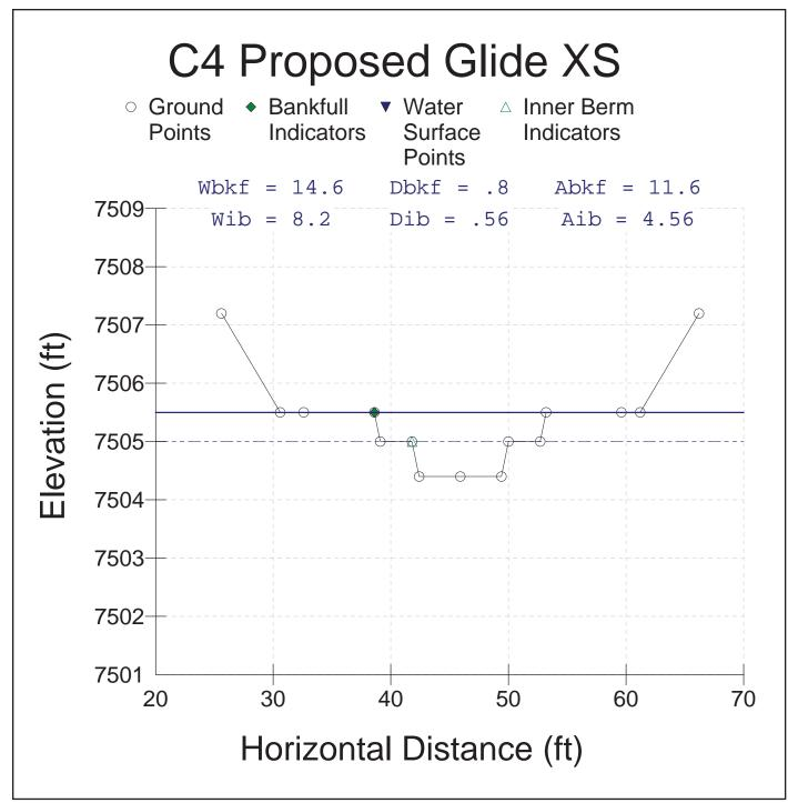
Figure 51. The typical *glide* cross-section for the proposed C4 reach below the West Creek road.
