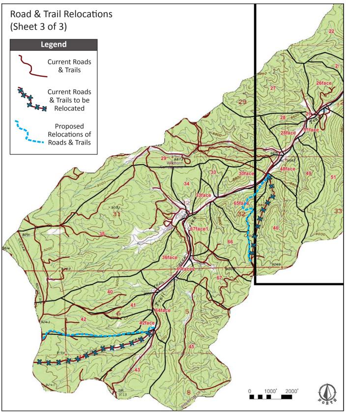
Figure 32. The proposed relocations of the problematic roads and trails illustrating the area in "Sheet 3" in Figure 29.
