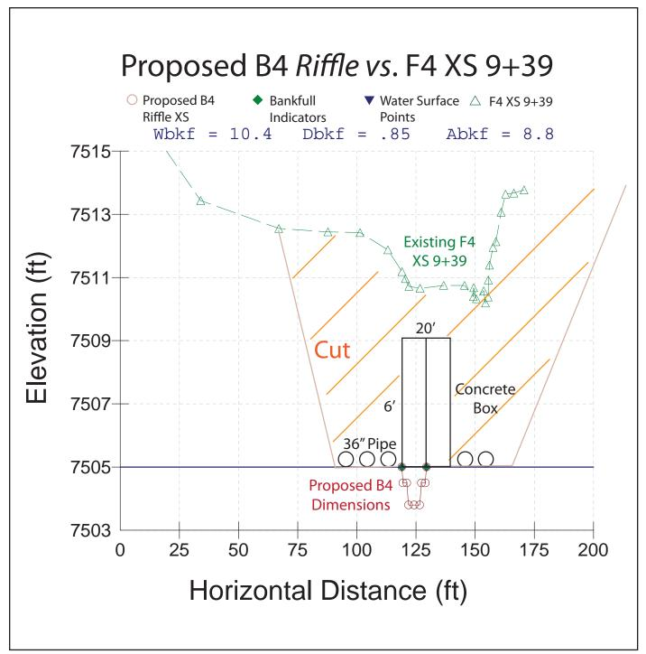
**Figure 66.** The proposed B4 *riffle* cross-section compared to the existing F4 cross-section 9+39, indicating the substantial excavation required.
