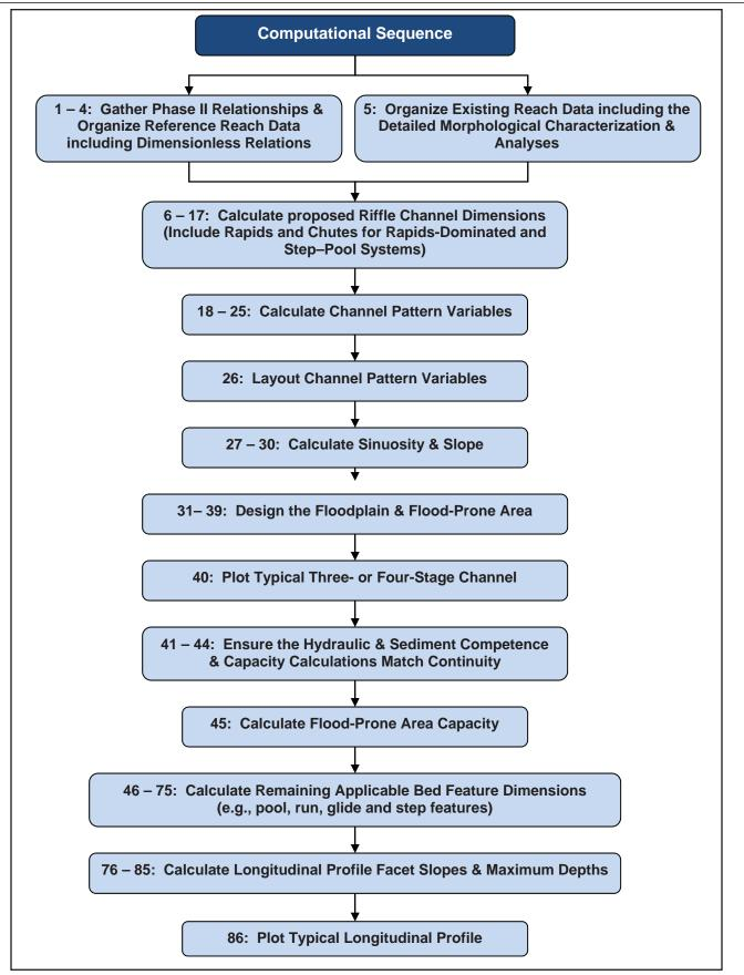
**Flowchart 2.** Computational sequence to determine and evaluate the dimension, pattern & profile variables for the proposed design reach.
