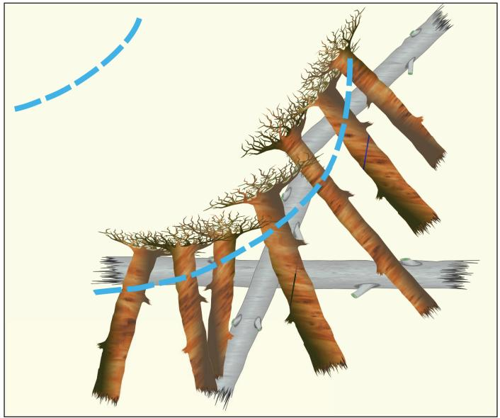
**Figure 14.** Plan view of toe wood placement prior to transplanting sod mats and woody vegetation (flow is left to right).
